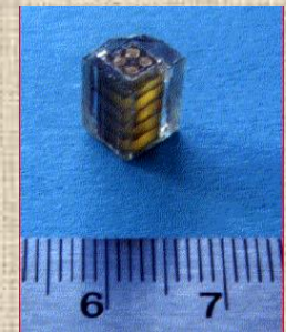
Transducer stack for ultrasonic sonar application (TRS Ceramics)
